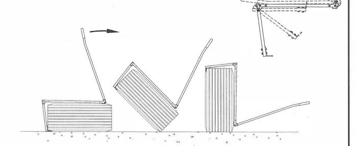
3. Engage the Wheel Hook under the outside of the tire. With the tool on the centerline of the tire, place the heel of the Rear Pivot Brackets on the opposite sidewall. Place one foot on the tire near the Pivot Brackets and pull back on the handle until the tire rotates to a vertical position.
